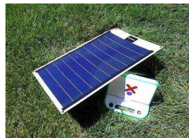
Example of a US$ 26, Thin-Film 10 watt solar panel from Gold Peak. Our involvement with the OLPC movement in the Pacific led to their solar panel manufacturer in China who then produced custom panels for SIL. 20 watt panels sold to members for US$ 75, or approximately $3.75 per watt (landed cost).
