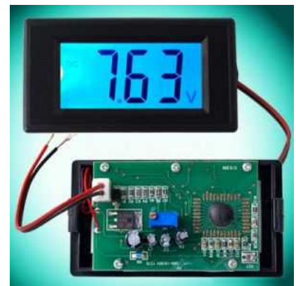
An inexpensive digital panel volt meter that can be mounted just about anywhere in the solar system. Be sure to find a 'self-powering' model.
