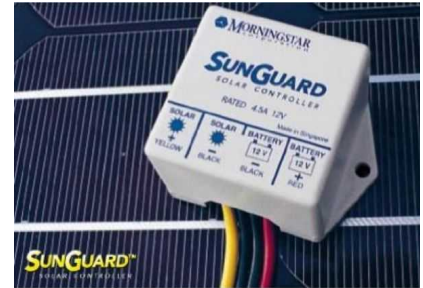
Inexpensive Morningstar Controller which could be used with a suitable alarm circuit, save costs. 4.5 amps can handle a 50 watt solar panel.
