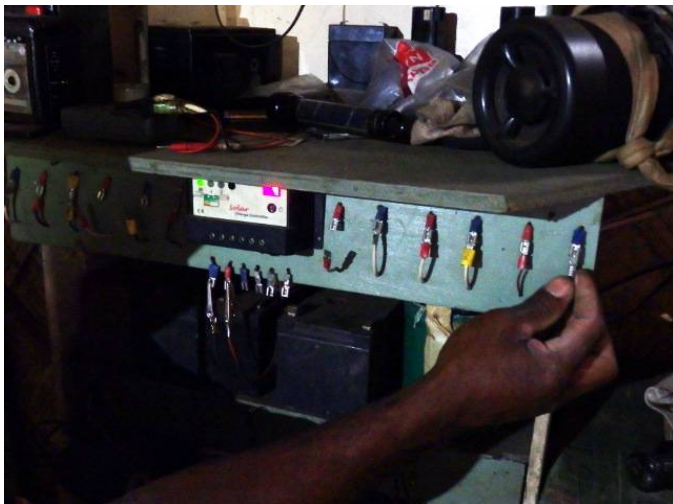
Andy, figured out this array of "switches" from crimp-on auto-connectors. He can direct power from the controller to separate batteries, and also control independent lights, by manipulating connectors.
